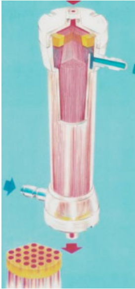
Figure 18.5 Cut out of a hollow-fiber dialyzer.
