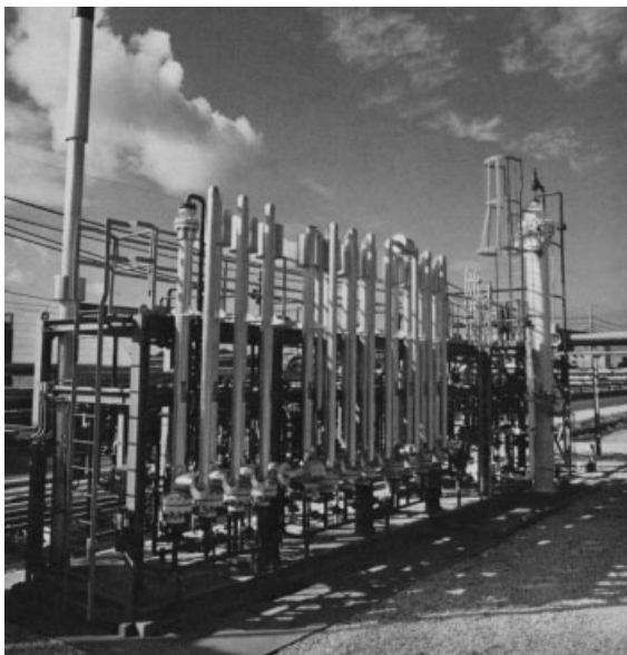
Figure 8.8 Photograph of a Permea hydrogen recovery unit installed at an ammonia plant. The hollow fine fiber modules are mounted vertically [6].
