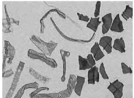
Fig. 8.6 X-ray absorption image showing separation of aluminum alloys based on the average atomic number of each particle. Courtesy of the Technical University of Delft, The Netherlands (see Acknowledgments)
