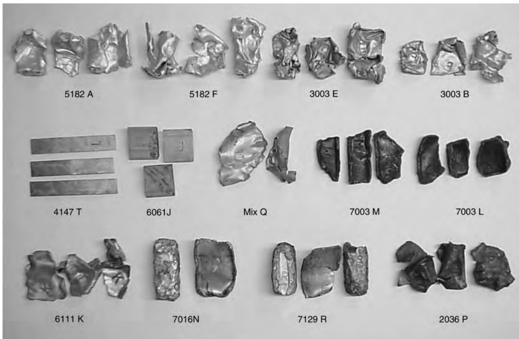
Fig. 8.3 Tint-etched shredded particles of known wrought aluminum alloys
