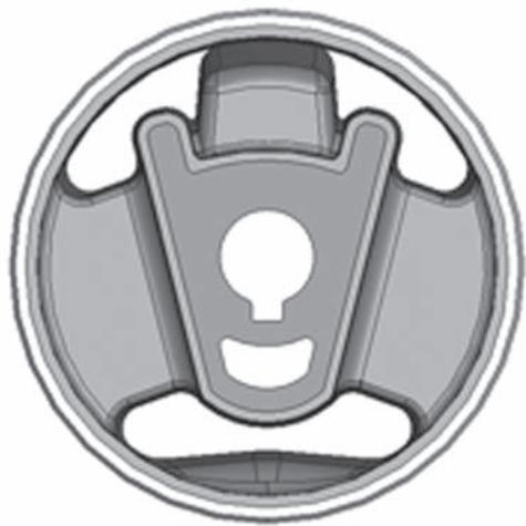
Figure 1. Typical suspension bushing with elastic springs and bump stops, outer sleeve and inner part.
