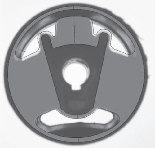
Figure 8. Suspension bushing after swaging. Front section of the FEM-model over the prototype.
