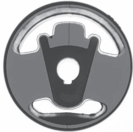
Figure 7. Suspension bushing before swaging. Front section of the FEM-model over the prototype.
