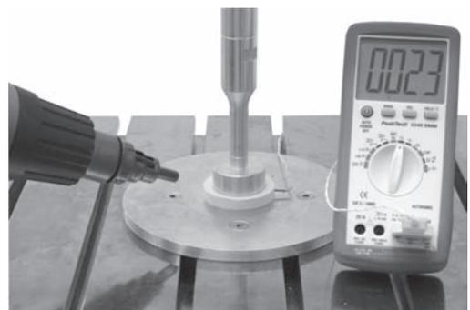
Figure 3. Adapted hydraulic impact test with heat gun and temperature sensor.
