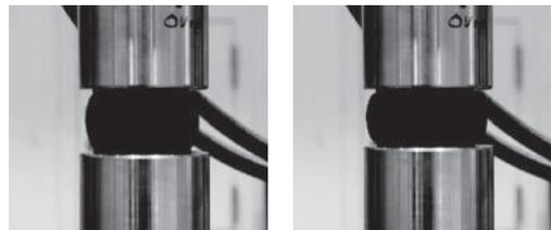
Figure 2. Test setup and load application. The rubber component, i.e. rubber cylinder and steel plates, is in the middle and the parts at the top and bottom are the fixtures used for controlling the rotations at load application. Load: 3 kN left and 5 kN right.
