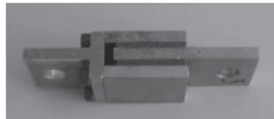
Figure 1. Simple shear MS rubber sample.
