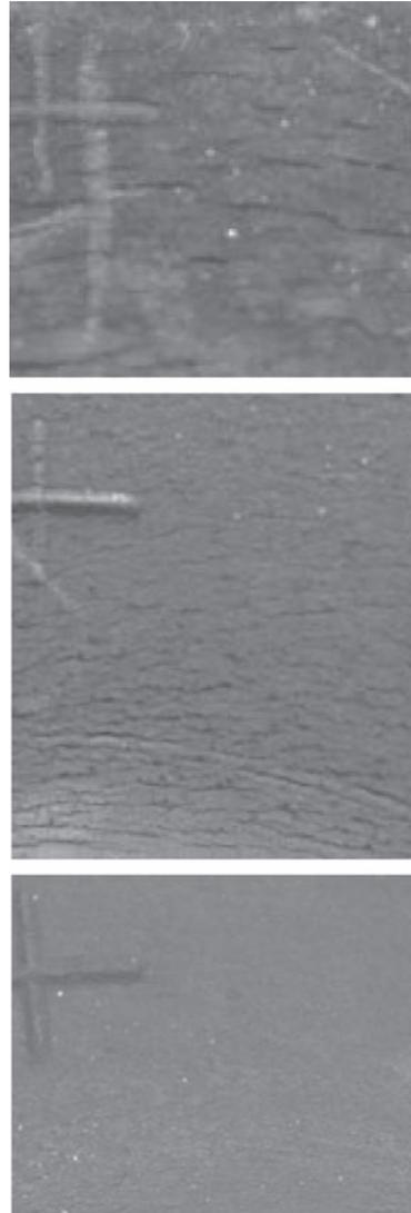
Figure 8. Comparison of component's surface after testing/service: service part (upper picture), tested part with ozone (middle picture) and tested part without ozone (lower picture).
