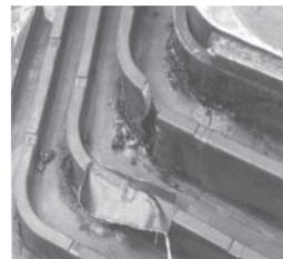
Figure 2. A metal failure of the Chevron rubber spring (after 0.7 million cycles).
