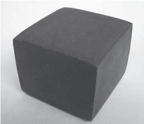
Figure 9. NR specimen after relaxation test (30 days at 353 K).
